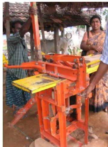
Semi-automated manufacture of soil-cement bricks and blocks (Kanyakumari & Pondicherry India)
