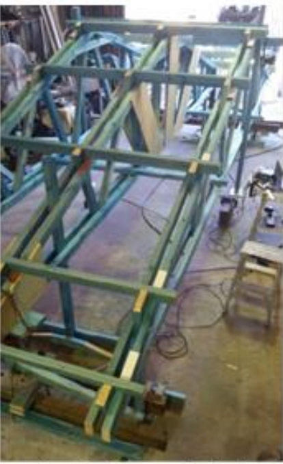
Two Test Trusses Pushed Up By Loading Truss
