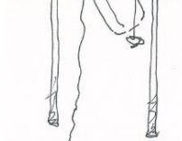
Fill container with water; screw on lid and hang container. Tie on soap.
