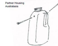
Partner Housing Australasia Heat the nail and make one water outlet hole and one air intake hole in the water container.
