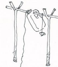
Fill container with water; screw on lid and hang container. Tie on soap.
