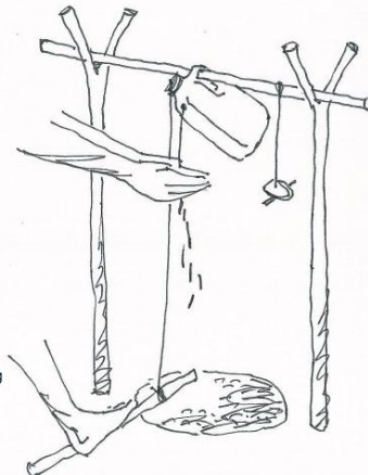
Make 300 – 400mm diameter soak pit below tap to prevent the tap location from becoming a mud hole and mosquito breeding place. Fill with gravel.
