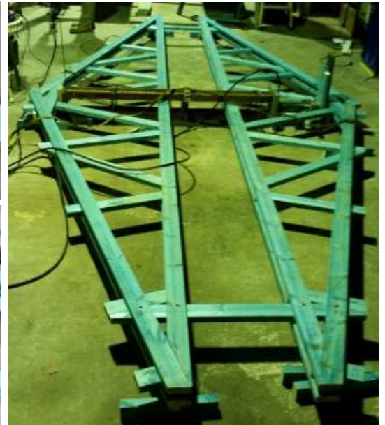
Two Test Trusses Being Pushed Apart
