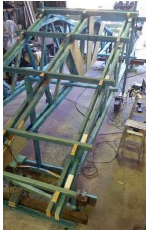
Two Test Trusses Pushed Up By Loading Truss
